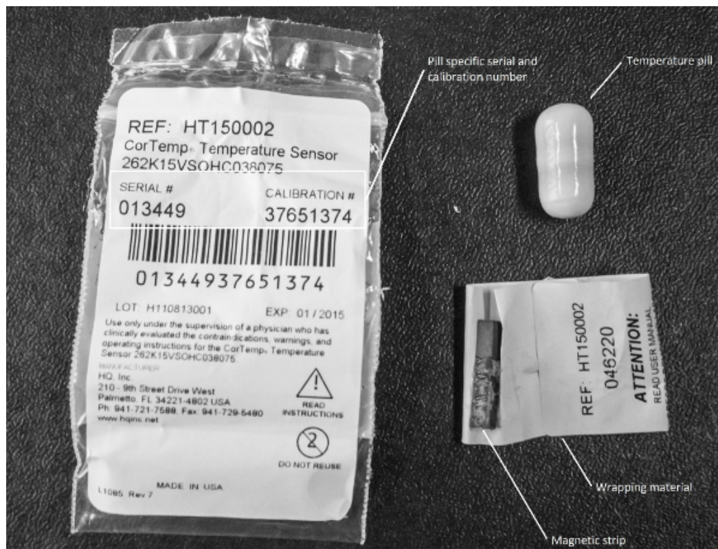
Figure 2. Ingestible telemetric temperature pill. Ingestible telemetric temperature pill and packing material. On the left the wrapping material is visible, which contains the temperature pill individual serial and calibration number. On the right, the temperature pill and the magnetic stripe are shown. In this case the temperature pill is not in contact with the magnetic stripe, which means that the battery is activated. Please click here to view a larger version of this figure.
